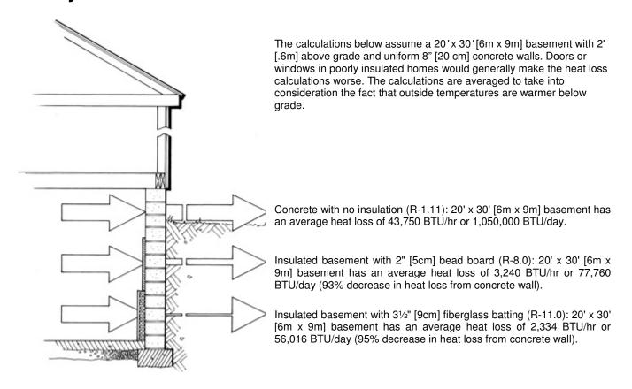
Adding even a modest layer of insulation to your basement walls will result in an incredible reduction in heat lost through the concrete walls. The results will be felt immediately - both in less fuel used and in more heat in the home.
