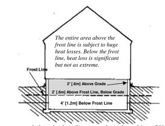
Temperatures below the frost line are relatively stable at 50°F [10°C] Heat loss is rapid right down to the frost line.
